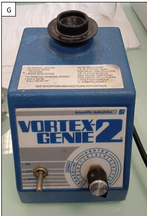
(Fig.E) Precision Balance - (Fig.F) Magnetic Stirrer at controlled rpm and T – (Fig.G) Oscillator Mixer - (Fig.H) Precision Rheometer “Anton Paar MCR 302”.
