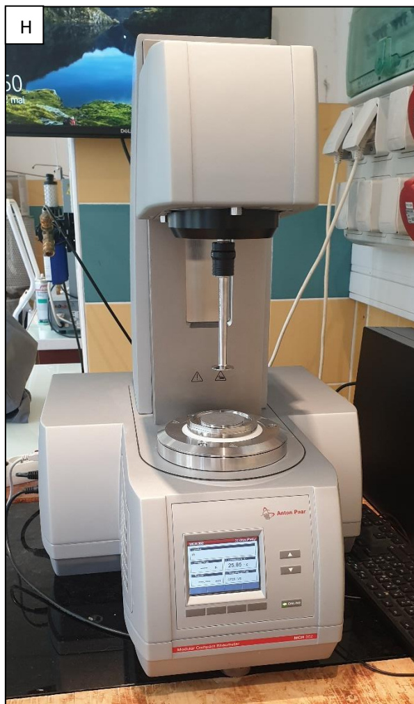
(Fig.E) Precision Balance - (Fig.F) Magnetic Stirrer at controlled rpm and T – (Fig.G) Oscillator Mixer - (Fig.H) Precision Rheometer “Anton Paar MCR 302”.
